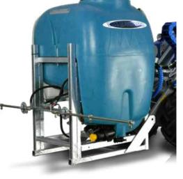
Street Washer is equipped with two foldable nozzle bars for street cleaning and a hand held washing gun with 10 m (32 ft) hose. The tank is equipped with a level indicator, a filter and a small separate water tank with a tap useful for wash the hands.
