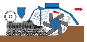
the rear field roller. With the optional seeding unit you are able to make a ready lawn surface on one pass. Stone burier is most commonly used when the topsoil needs to be milled thoroughly.
